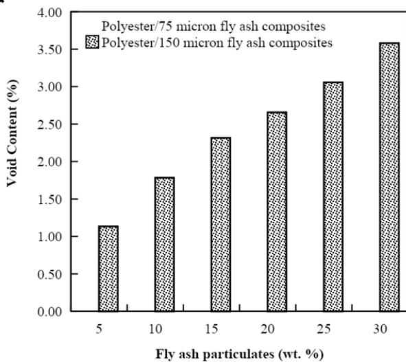
Fig. 2 Void content generated in polyester composites filled with different particle size of fly ash
