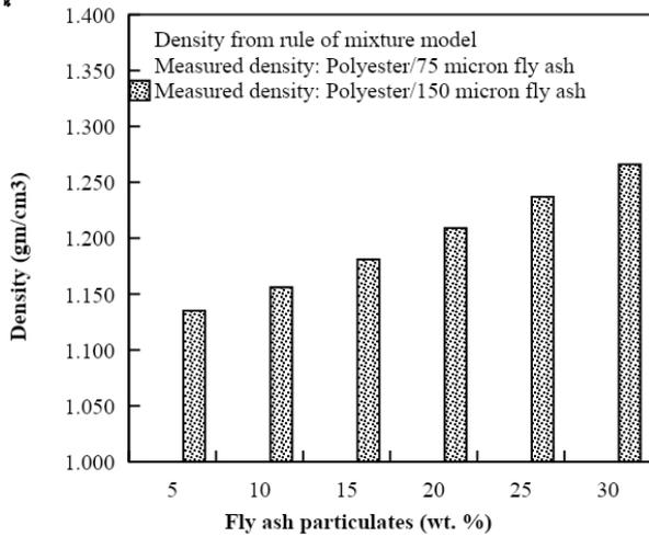
Fig. 1 Measured and calculated density of polyester filled with different particle size of fly ash
