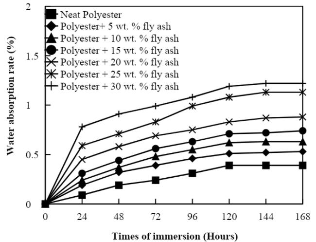
Fig. 3 Water absorption rate of polyester composites filled with fly ash of 75 microns particle size
