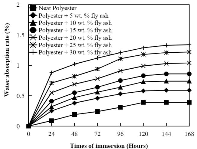
Fig. 3 Water absorption rate of polyester composites filled with fly ash of 150 microns particle size
