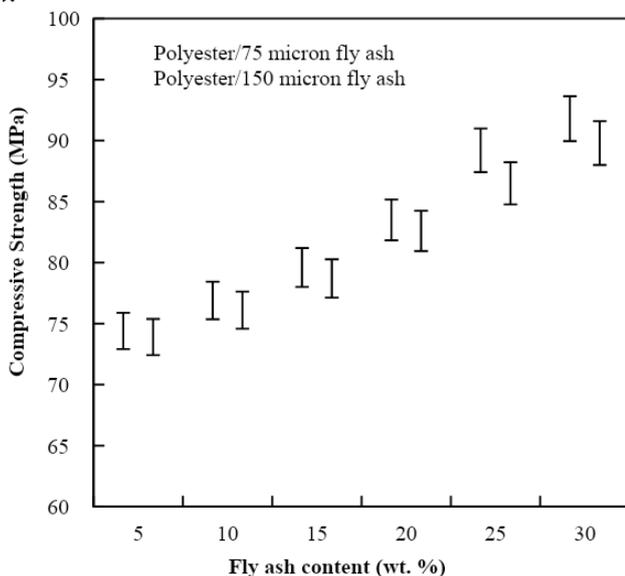
Fig. 3 Compressive strength of polyester filled with different particle size of fly ash
