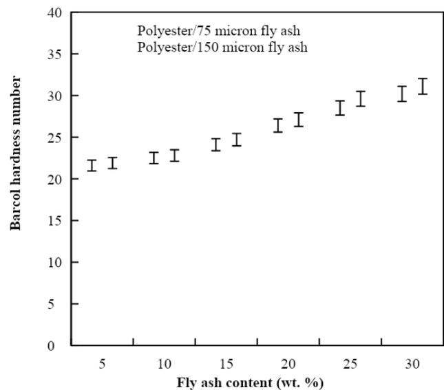
Fig. 3 Hardness of polyester filled with different particle size of fly ash
