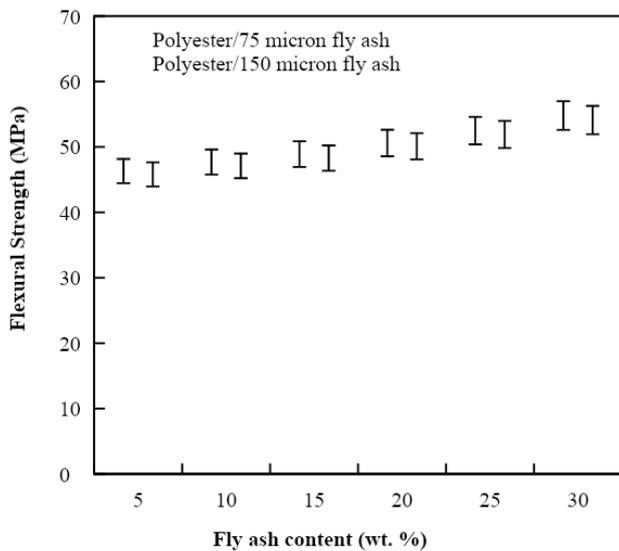
Fig. 2 Flexural strength of polyester filled with different particle size of fly ash
