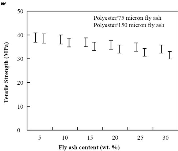
Fig. 1 Tensile strength of polyester filled with different particle size of fly ash
