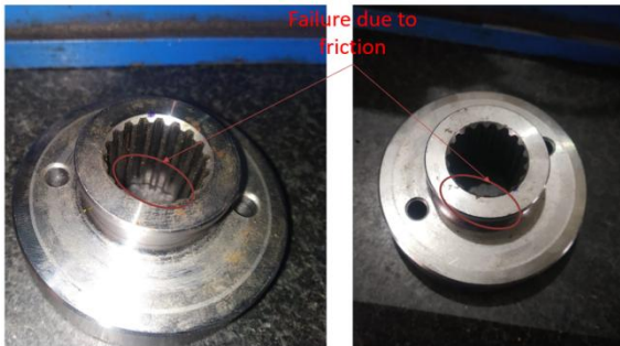
Figure 1 Failure due to friction
