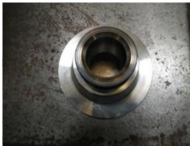
Figure 7 After lathe operation
