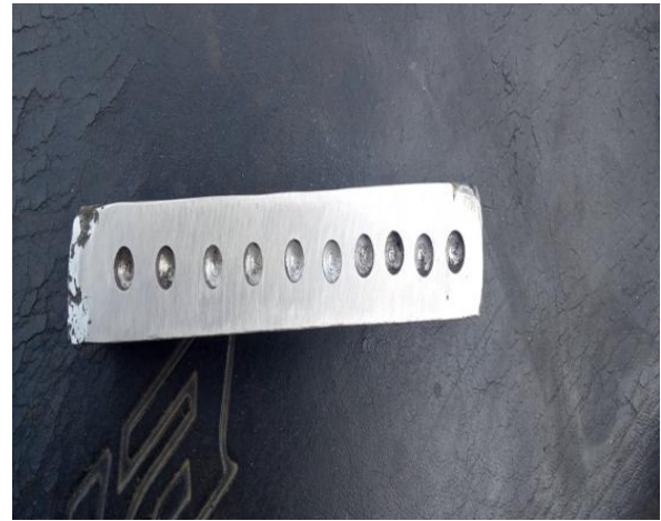
Fig.3. Specimens of WEDM Machined
