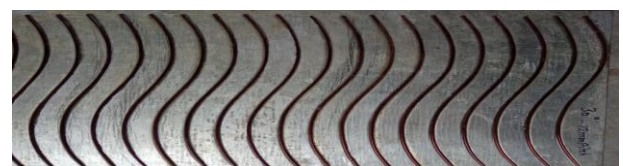
Fig. 2.4 Roughened Plate with 12mm pitch and 30° arc angle
