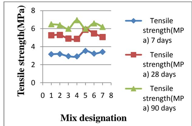
**Fig2:Split tensile strength graph**
